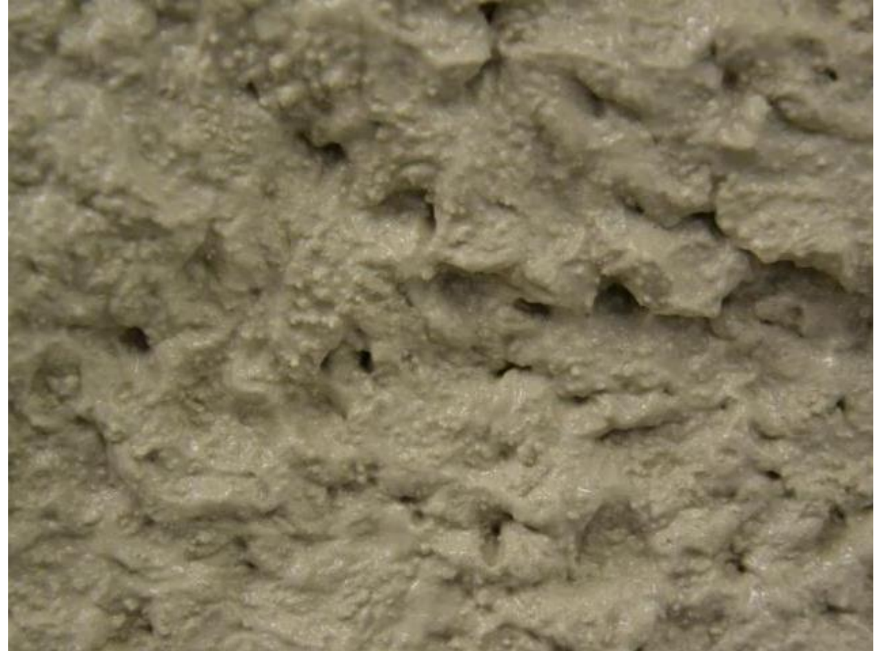
Close-up, fresh mortar, \rho_{\text{fresh}} \sim 350 \text{ kg/m}^3
