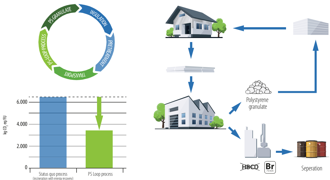
Figure 18 Recycling process within the PolystyreneLoop from demolition waste to new insulation boards; Principle of PolystyreneLoop with Bromine recovery unit
