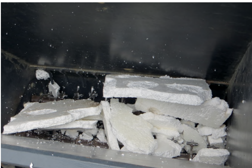
Figure 19 To significantly reduce the volume of insulation waste for transportation and storage before recycling treatments, mobile units to be used at demolition sites have been developed. ©Ralf Pasker
