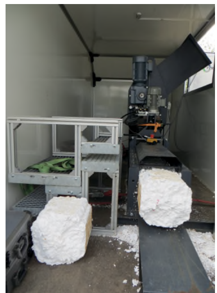
Figure 19 To significantly reduce the volume of insulation waste for transportation and storage before recycling treatments, mobile units to be used at demolition sites have been developed. ©Ralf Pasker
